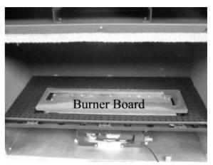
Single layer of Pebbles over burner Avoid placement of pebble shaped over pilot head
